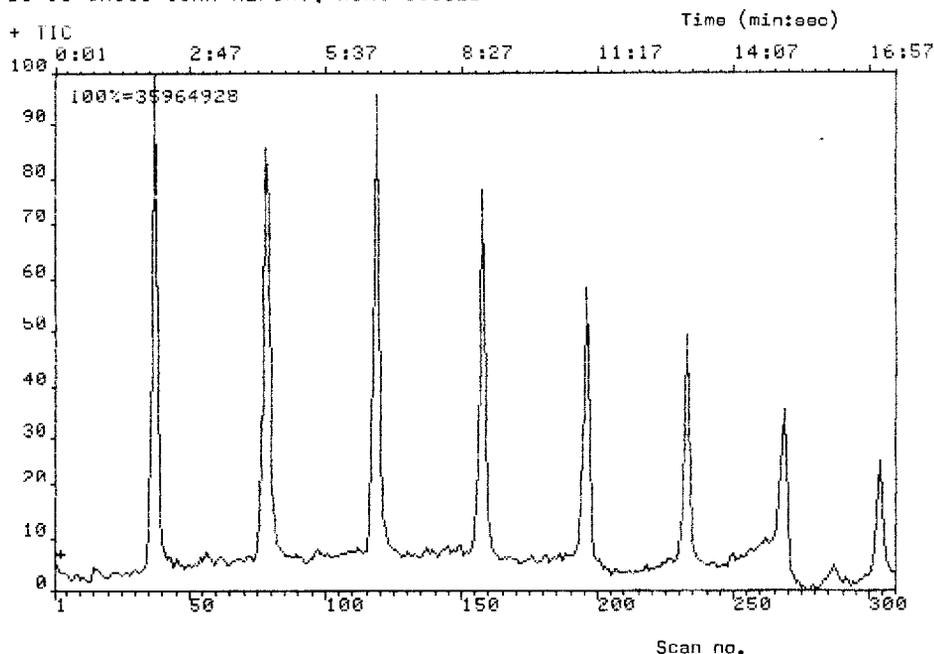
Fig. 5. Part of the total ion current trace of a GC-MS analysis of mixture of *n*-alkanes up to  $n\text{-C}_{54}\text{H}_{110}$ . These are the raw data. No background subtraction has been performed.
