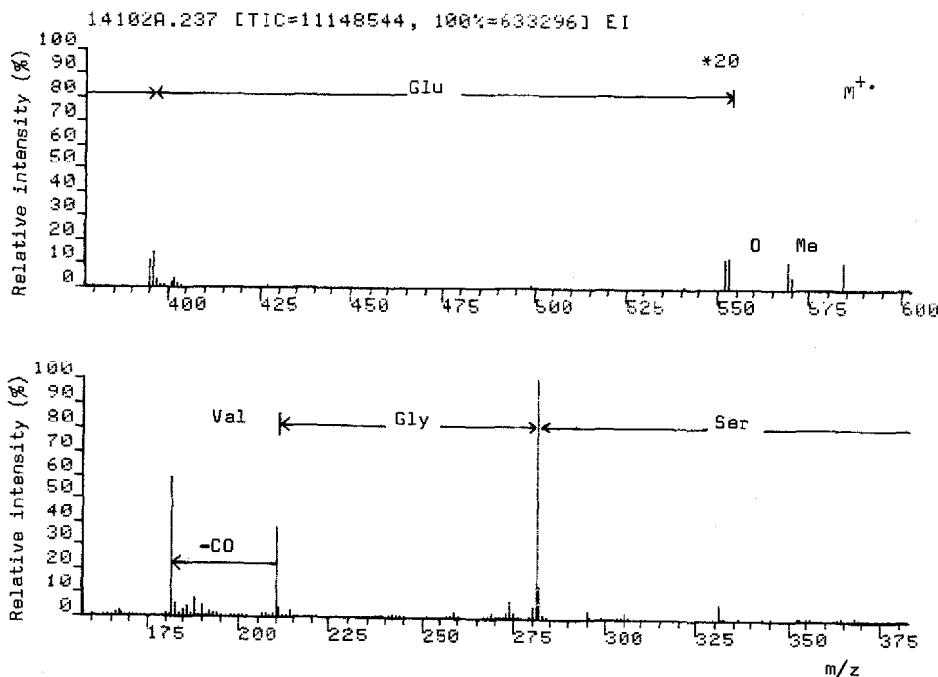
Fig. 4. Mass spectrum of Val-Gly-Ser-Glu obtained using the direct coupling schematized in Fig. 1. No silylation was necessary since the column extends into the ion source. There is less fragmentation than in Figs. 2 and 3, *i.e.* more relative intensity in the fragments of higher mass. The non-sequence ion at  $m/z$  193 is no longer prominent. An amount of derivative corresponding to 500 pmol of peptide was injected.
