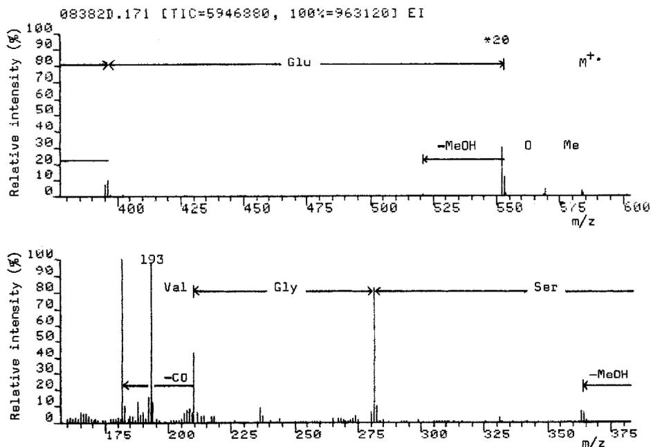
Fig. 2. Mass spectrum of Val-Gly-Ser-Glu obtained using the commercial (jet-separator) interface. An amount of N<sup>ε</sup>-trifluoroacetyl-N,O-permethyl derivative corresponding to 1 nmol of peptide was injected. Although the interface had been treated with Silyl-8, the mass spectrum shows evidence of excessive fragmentation, in particular the ion at *m/z* 193.
